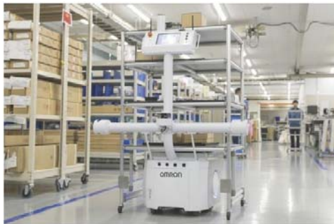
Autonomous mobile robots can self-navigate throughout a facility using onboard mapping software. Courtesy: Omron Automation Americas
