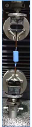
Slip Test Underway
