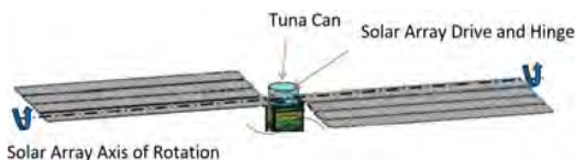
Figure 1: Deployed SADA [IPSP 2014]
