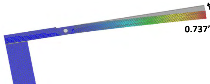
Figure 3: FEA Results of Max Deflection
