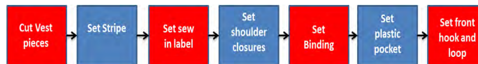
Figure 2: Visual of Vest Workstations, in red, that should have accumulated WIP inventory during EOY count
