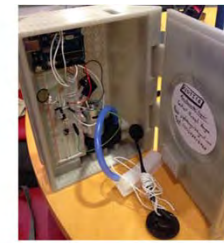
Figure 5: Hard shell housing case compatible with wheelchair
