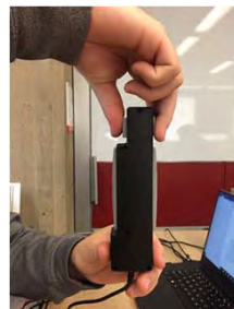
Figure 3: Dynamometer device used to test pinching force
