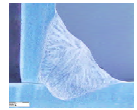
Figure 3: Micrograph of a MIG Weld
