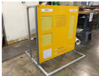
3'x3' Mockup Radar Cabinet Assembly
