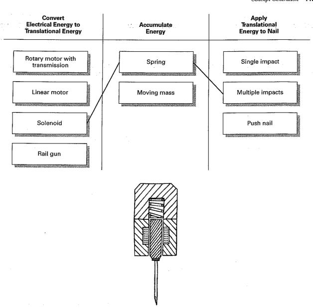
**EXHIBIT 6-10** In this solution concept, a solenoid compresses a spring and then releases it repeatedly in order to drive the nail with multiple impacts.
