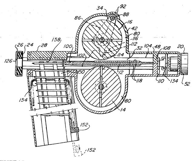
**EXHIBIT 6-5** Concept from motor-driven double-flywheel nailer patent (U.S. Patent 4,042,036). The accompanying text describing the patent is nine pages long.
