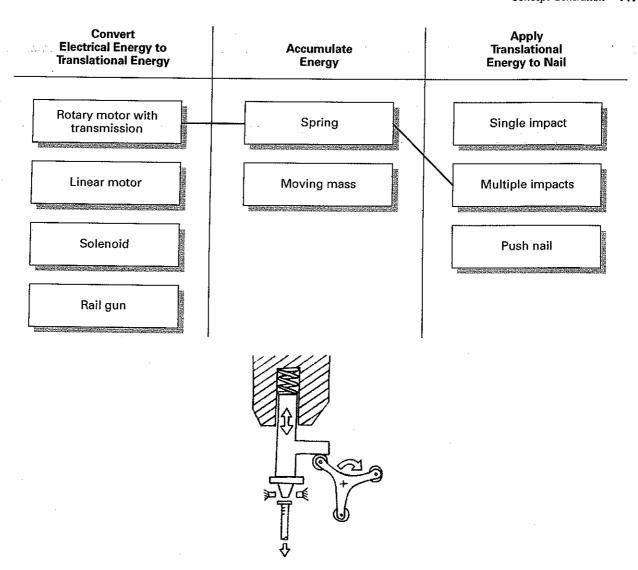
**EXHIBIT 6-12** Solution from the combination of a motor with transmission, a spring, and multiple impacts. The motor repeatedly winds and releases the spring, storing and delivering energy over several blows.
