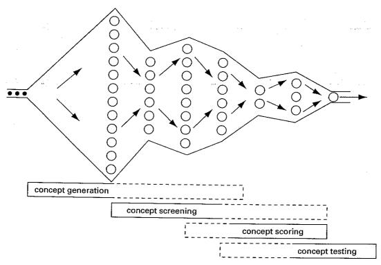
**EXHIBIT 7-4** Concept selection is an iterative process closely related to concept generation and testing. The concept screening and scoring methods help the team refine and improve the concepts, leading to one or more promising concepts upon which further testing and development activities will be focused.
