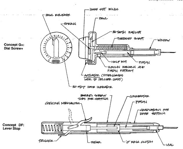
**EXHIBIT 7-6** New and revised concepts for the syringe. During the selection process, the syringe team revised concept G and generated a new concept, DF, arising from the combination of concepts D and F.
