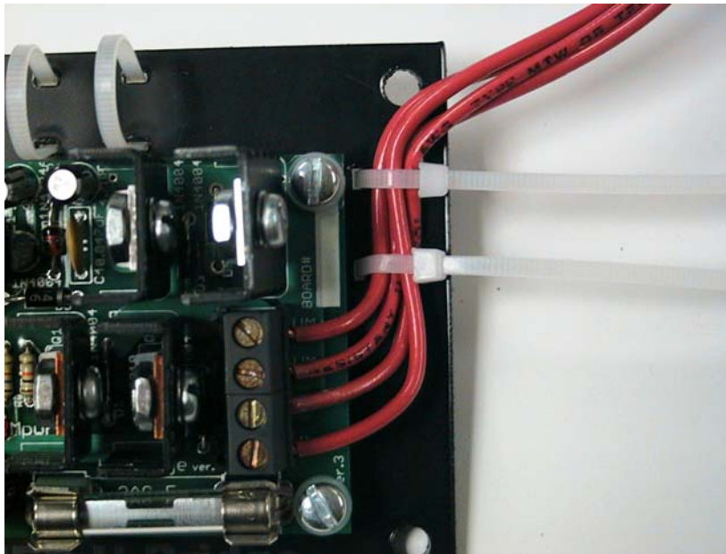
Partial view of H-bridge board backer and strain reliefs
