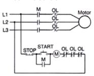
A magnetic starter contains a mechanism for opening and closing a set of contacts in the motor circuit and a thermal overload protective device. When the coil is energized, movable contacts complete the electrical circuit. De-energizing the coil opens the circuit. Magnetic starters are frequently controlled by pushbutton, limit switches, relays, timers, pressure switches, and float switches.
