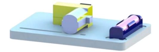
Figure 16: The base subassembly with the motor and battery cover glued in place
