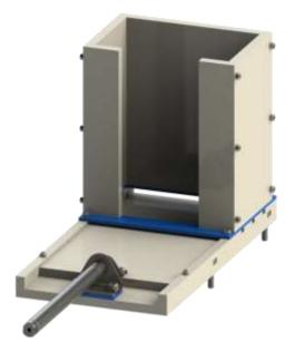
Figure 22 - Lower Base Escapement Feeder & Slider
