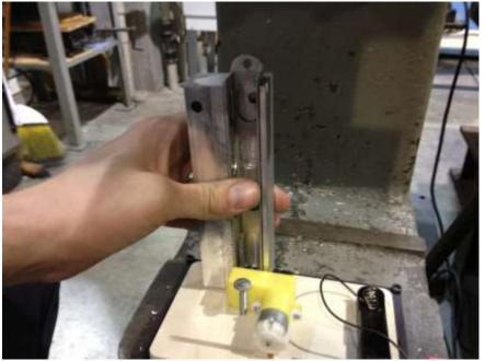
6. Slowly lower the press fixture looking through the slot on top to make sure the Arc of the top of the channel is aligned. The arc should be aligned to the top left of the slot.
