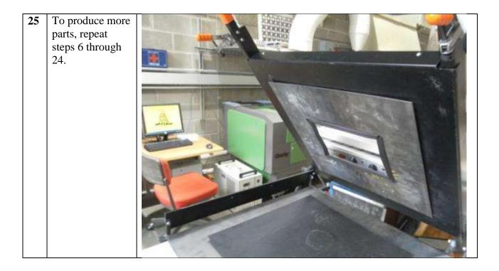
When the part is finished molding, remove the material and mold. Return any excess materials to their respective homes.
