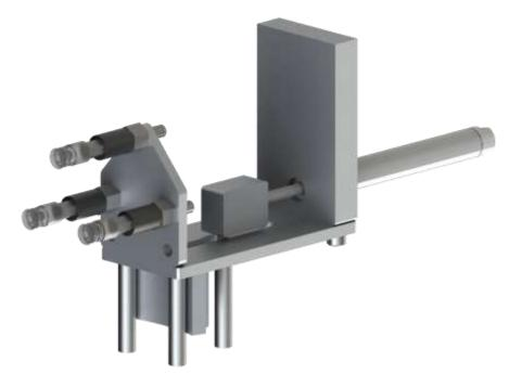
Figure 31 - Gripper/Suction End Effector
