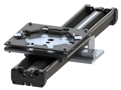
Figure 26 - Ultrasonic Welding Slider
