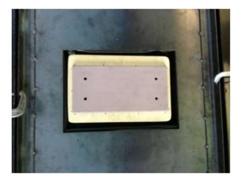
4. Place .06" inch thick polystyrene sheet on top of rubber siding and clamp down using the 2 orange vices. Make sure rubber moulding doesn't get in the way.
