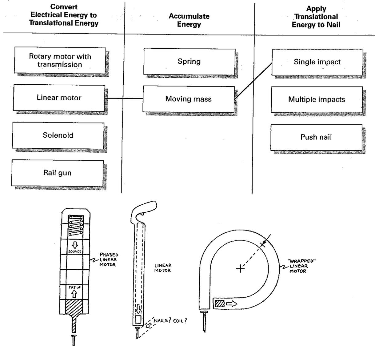
**EXHIBIT 6-13** Solutions from the combination of a linear motor, a moving mass, and single impact. A linear motor accelerates a massive hammer, accumulating kinetic energy which is delivered to the nail in a single blow.
