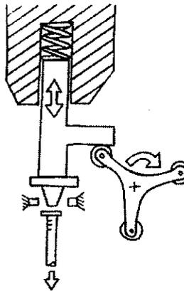
**EXHIBIT 6-12** Solution from the combination of a motor with transmission, a spring, and multiple impacts. The motor repeatedly winds and releases the spring, storing and delivering energy over several blows.
