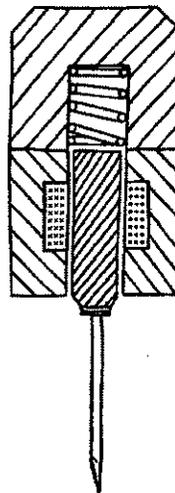
**EXHIBIT 6-10** In this solution concept, a solenoid compresses a spring and then releases it repeatedly in order to drive the nail with multiple impacts.
