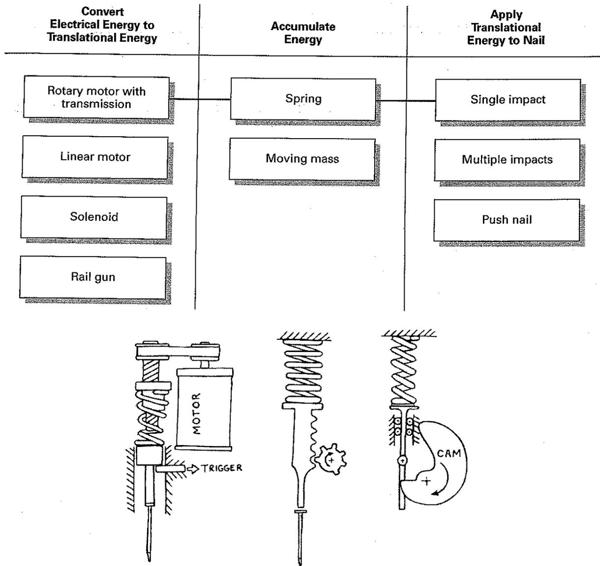
**EXHIBIT 6-11** Multiple solutions arising from the combination of a motor with transmission, a spring, and single impact. The motor winds a spring, accumulating potential energy which is then delivered to the nail in a single blow.
