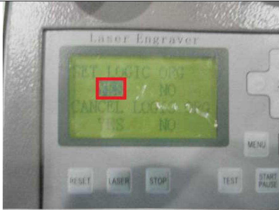
**16** Push the “ESC” button to exit the “LOGIC ORG” screen. The laser is now ready to run.
