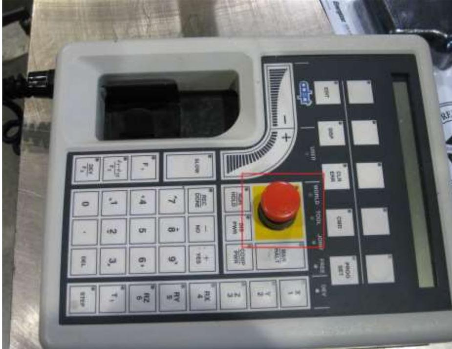
13 To re-engage the robot, turn the E-Stop button on the pendant clockwise until it clicks, then push the "COMP/PWR" button on the pendant.
