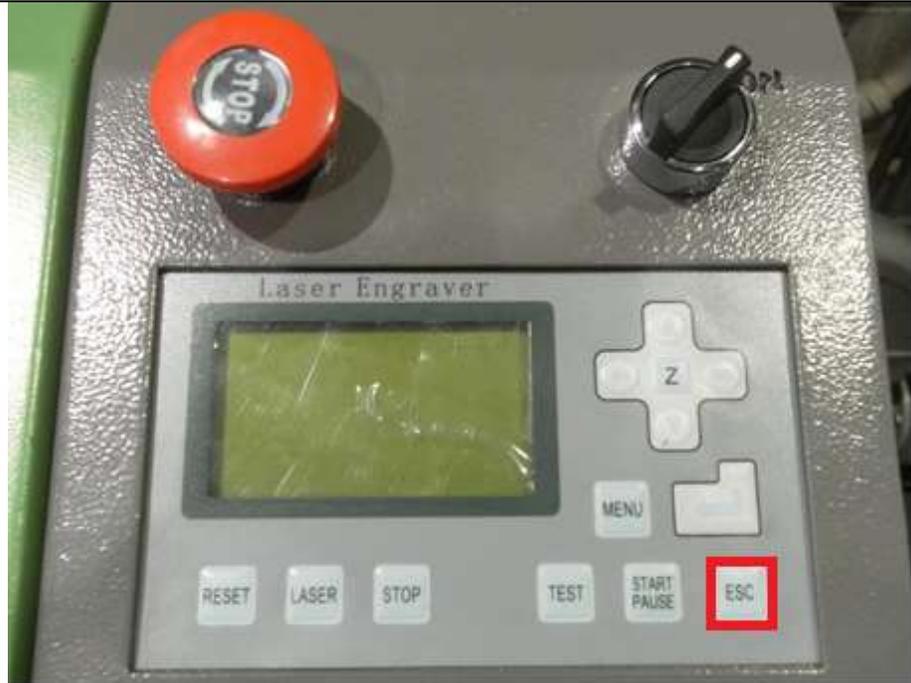
**12** Push the “Z” button in the middle of the arrow keys and then the “RESET” button to focus and set the Z axis. The laser is now ready to run.
