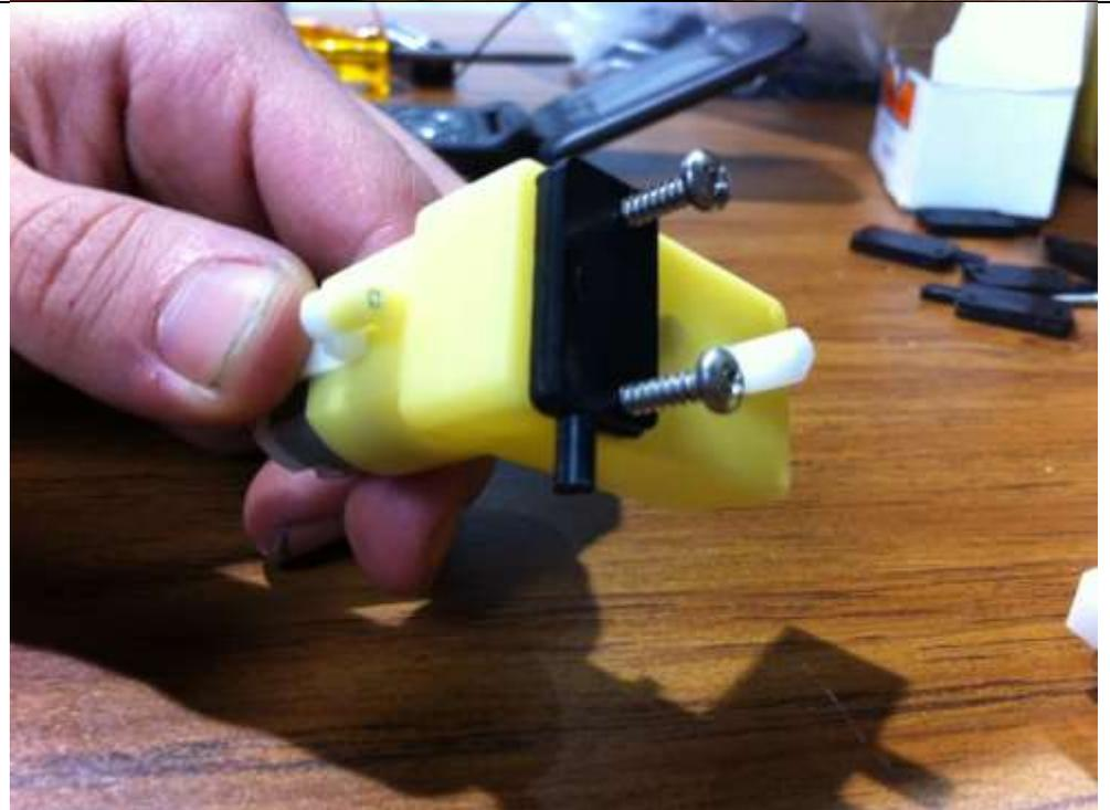
A close-up photograph showing a person's hands holding the yellow motor housing. A black motor strap is being attached to the side of the motor. Two screws are being inserted into the motor housing to secure the strap. The motor is resting on a wooden surface. |
