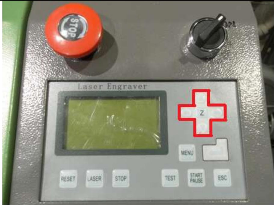
9 Push the “ENTER” button when the probe is positioned.
