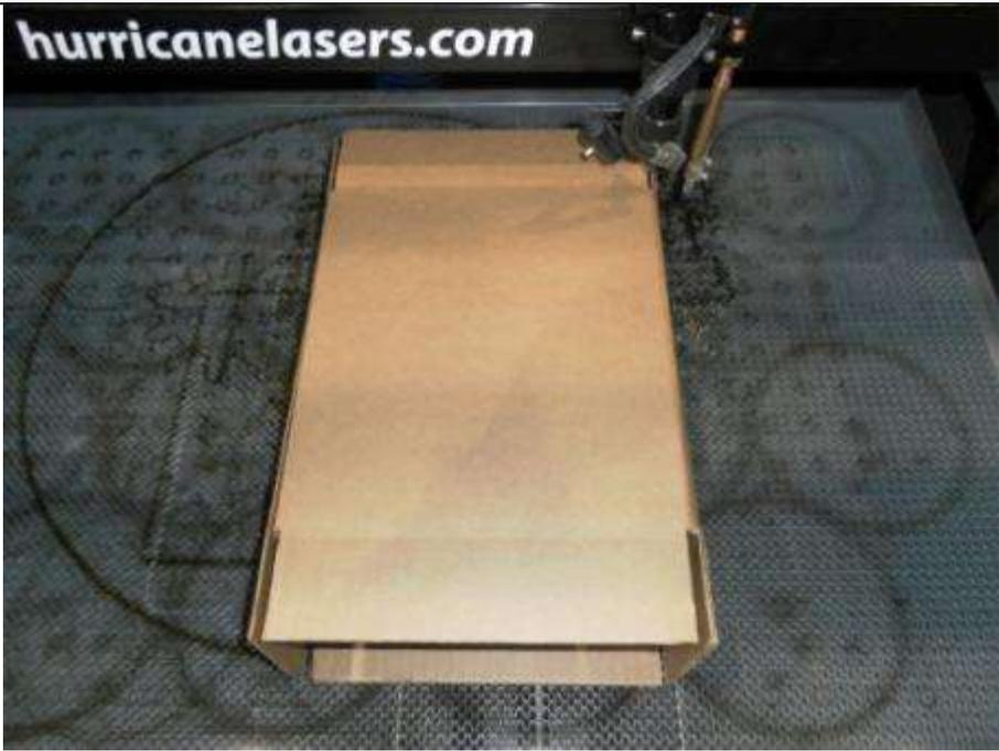
**26** Follow steps 17-24, this time opening the called "Box Back Optimized.e cp. Running this file will etch the back of the box as shown.
