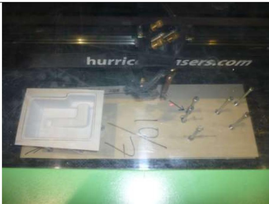
25 Remove the trimmed part from the left side of the fixture, and place it on the right side in the orientation shown, ensuring 3-point contact on the upper left corner (indicated by an arrow on the base of the fixture). Place a new part on the left side ensuring 3-point contact as before.
