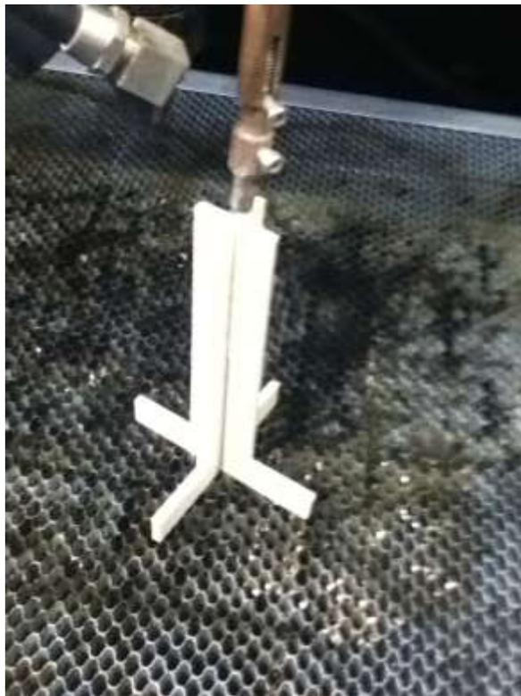
**9** Push the “Z” button in the middle of the arrow keys and then the “RESET” button to focus and set the Z axis.
