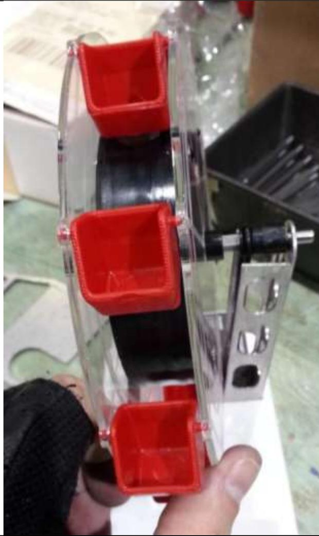
5 Then, insert the A-frame so that it sits in its groove in the lower base, and the axle slides through it. It is often easiest to slide it in at an angle, and then straighten it after it's in its groove.
