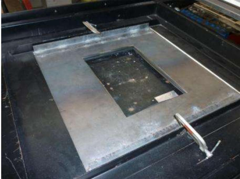
A photograph showing a rectangular metal mold plate being raised within a dark-colored machine. The plate is positioned in the center of the machine's frame, and a silver metal handle or lever is visible on the right side, likely used to operate the raising mechanism. |
