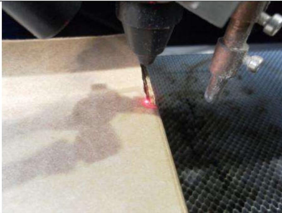
**14** Push the “ENTER” button when the probe is positioned.
