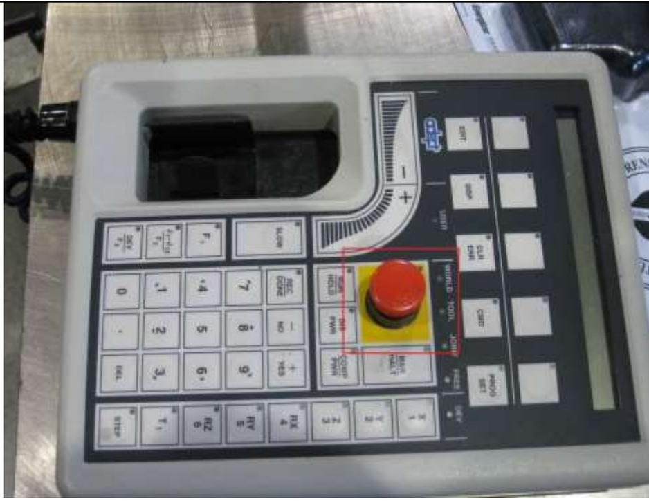
12 To re-engage the robot, turn the E-Stop button on the pendant clockwise until it clicks. Push the "COMP/PWR" button on the pendant.
