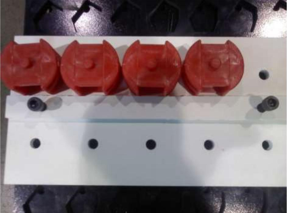
A photograph showing four red, dome-shaped dosers arranged in a row within a white plastic pallet. The pallet has several circular holes along its length. The dosers are positioned in the top row of the pallet.                                                                                            |
