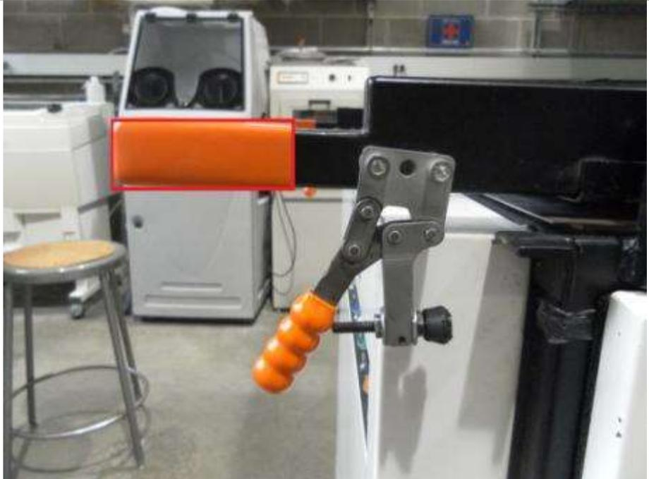
A photograph showing a holding fixture with two bright orange handles. The fixture is mounted on a white machine. In the background, there is a white cabinet with two circular openings, a metal stool, and other equipment in a workshop setting.                     |
