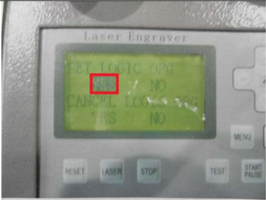
**11** Push the “ESC” button to exit the “LOGIC ORG” screen.
