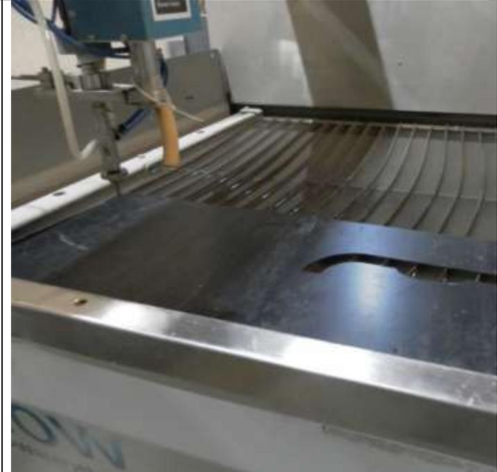
A photograph showing a dark, rectangular material placed on a curved metal grate within a waterjet cutting bed. The machine's nozzle and various hoses are visible in the background.                              |
