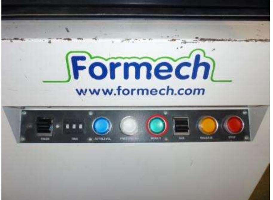
A photograph of the control panel of a Formech machine. The panel is white with the Formech logo and website address (www.formech.com) printed on it. Below the logo is a black control strip containing several buttons and switches: a black switch labeled 'TIMER', a black switch labeled 'TIME', a blue button labeled 'AUTOLEVEL', a white button labeled 'PRESSURE', a red button labeled 'MOULD', a black switch labeled 'AIR', a yellow button labeled 'RELEASE', and a red button labeled 'STOP'. |
