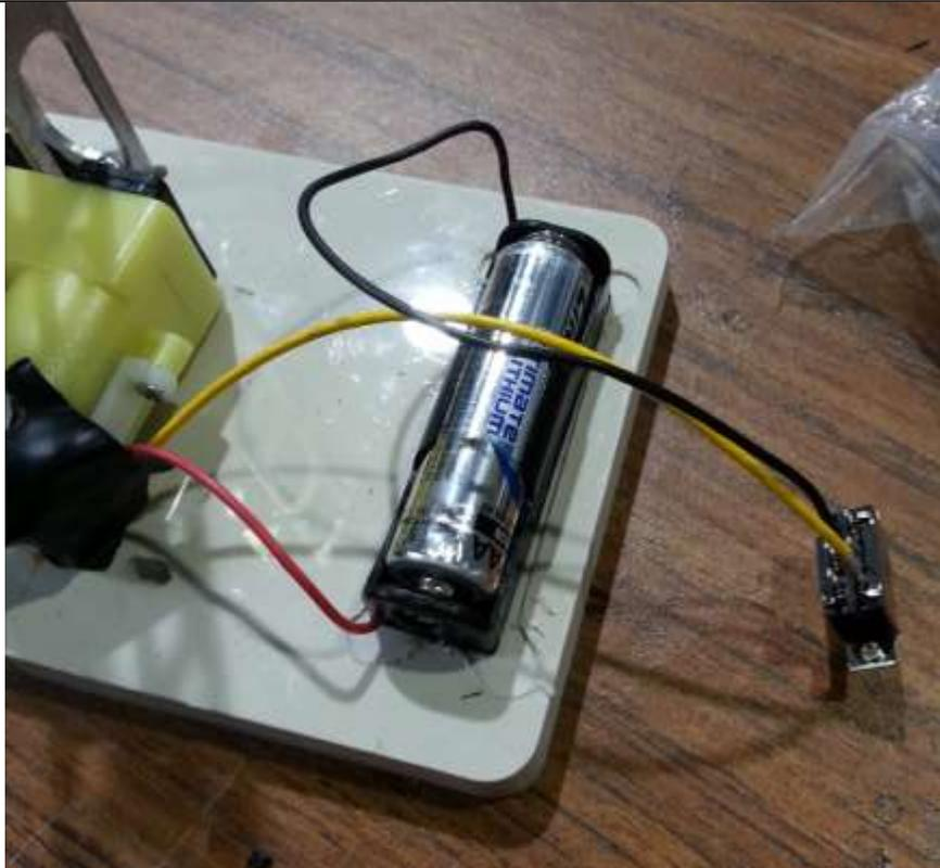
4 Flip the switch between the two positions, and ensure that the motor spins in one position and not the other. Also try to make sure that the motor spins in the correct direction; the motor should spin counter-clockwise when viewed from the front of the base.
