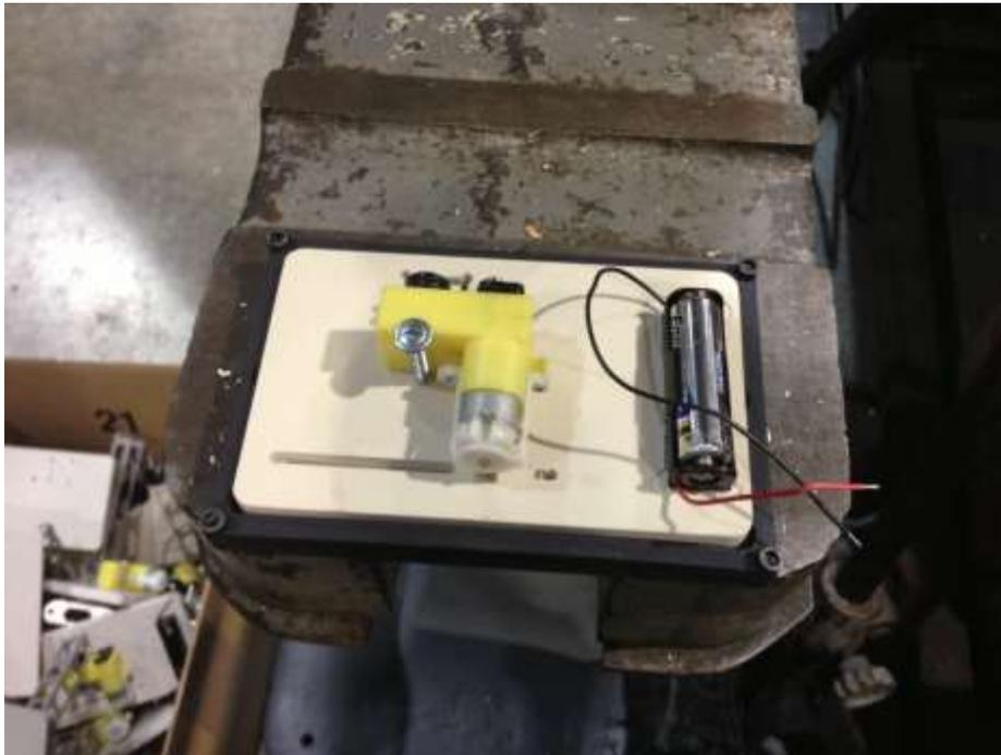
2. Make sure the base is fully inserted into Lower Press fixture and not sticking up.
