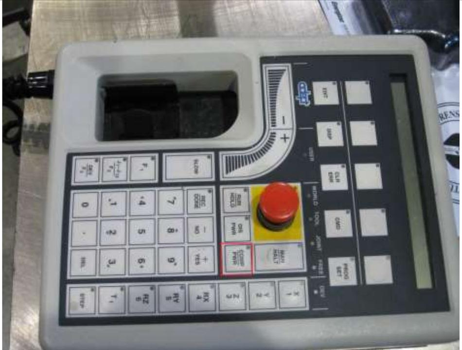
14 Push the flashing high power button on the control panel on the side of the base of the Adept workspace.
