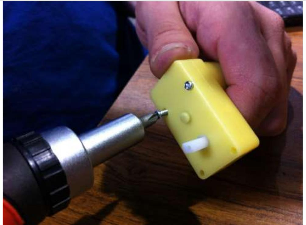
A close-up photograph showing a person's hands holding a yellow motor housing. A power drill with a silver bit is being used to remove a screw from the side of the motor. The motor is resting on a wooden surface.                                                  |
