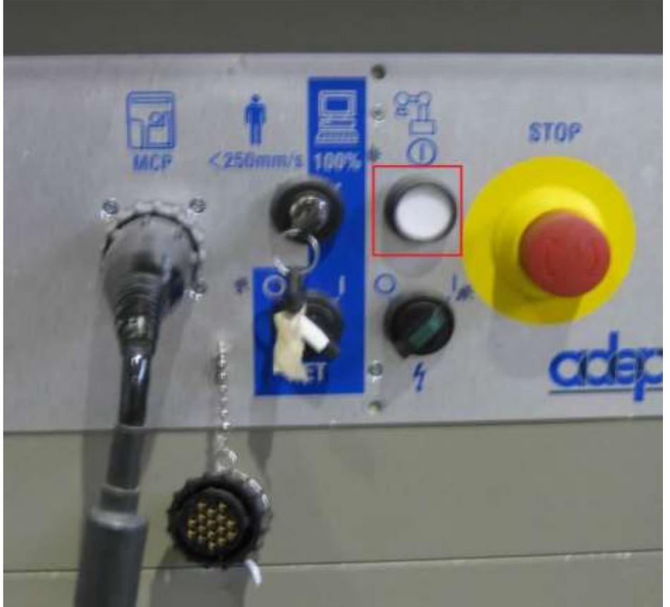
15 Once completed, the robot will pick and place the part on the conveyor. Remove the finished product and place it in the finished product receptacle. To end the cycle and shut off the machine, push the E-Stop button on the pendant.
