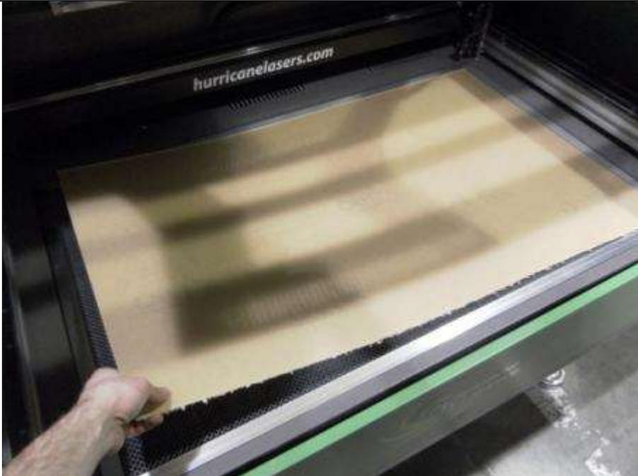
8 Used the arrow keys to position the focusing probe over the material. Define the origin to the upper right hand corner of the stock.
