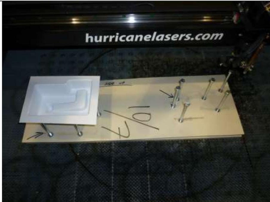
**24** Press "enter" on the machine several times to fully load the new program. Then press "Start Pause" to begin running the program. The program will cut the base out of its flashing; as soon as it is done press "stop" on the machine, while it is moving toward the right side of the fixture as shown.
