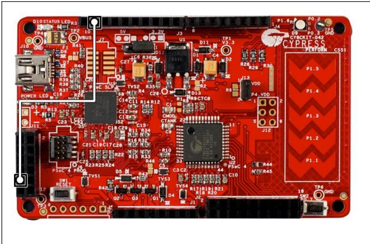
Figure 9: PSoC 4 Pioneer Kit UART TX Connection
